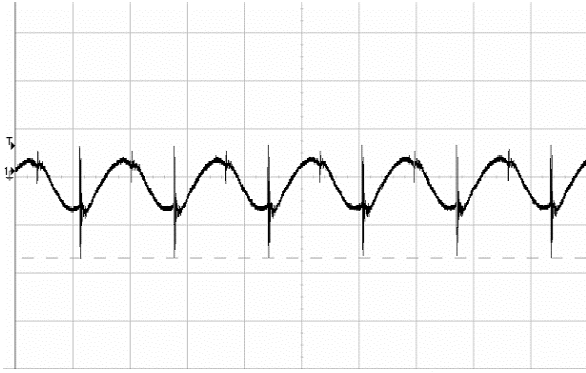
Figure 3 Output ripple & noise (2µs/div, 20mV/div), see Figure 15 for test configuration
