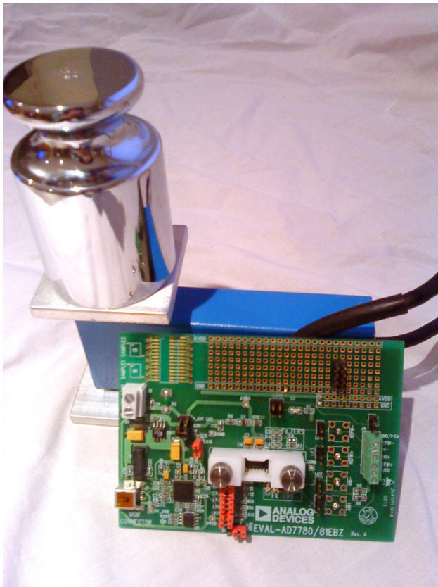
Figure 2. Weigh Scale System Using AD7781
