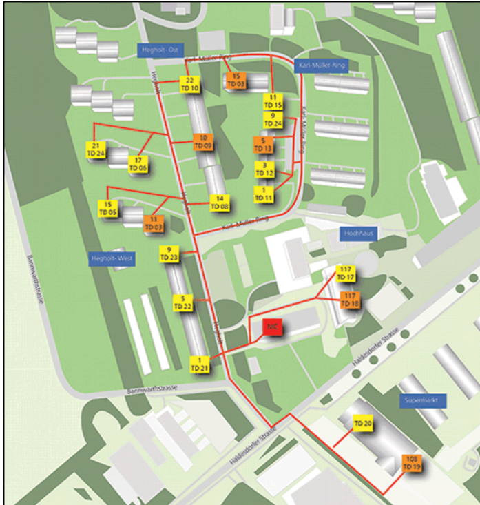
Figure 2. A typical environment of an urban grid with the maximum distance between nodes at 20m. Installation of one access node in a substation and installation of 22 nodes at one customer's premises. Image supplied courtesy of Devolo AG.
