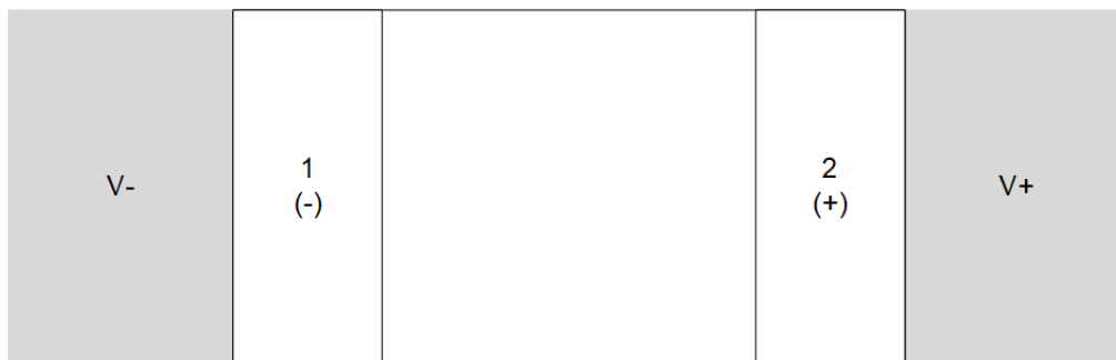
Figure 11-1. Recommended Layout: DEC Package
