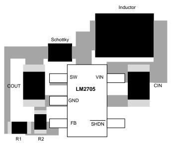
Figure 25. LM2705 Layout Example
