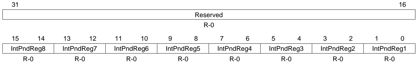
Figure 20-38. Interrupt Pending X Register (DCAN INTPND X) [offset = ACh]
