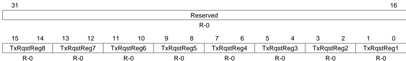
Figure 20-28. Transmission Request X Register (DCAN TXRQ X) [offset = 84h]
