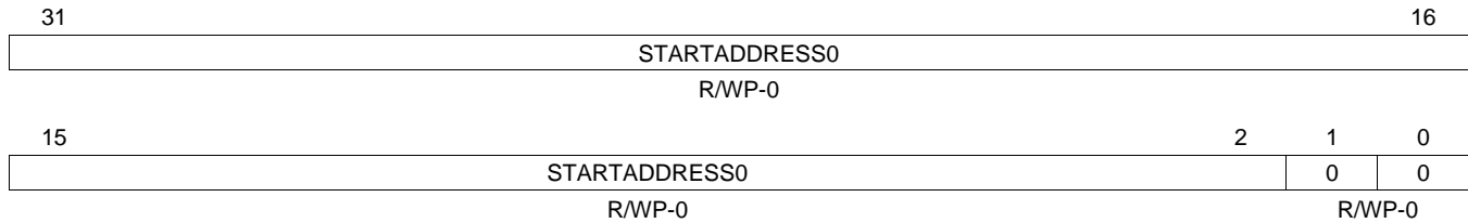
Figure 18-40. Memory Protection Start Address Register 0 (HTU MP0S) [offset = 74h]
