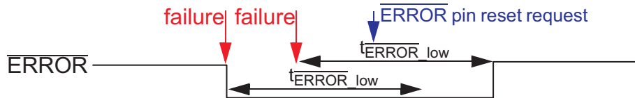
Figure 11-7. \overline{\text{ERROR}} Pin Timing - Example 4
